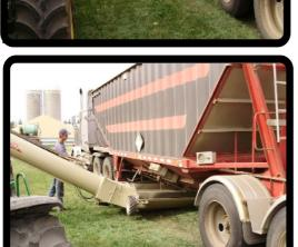
The Rodono Xtend Retracting Swingaway Hopper replaces the factory swingaway to allow the unloading of trucks of any configuration with out the need for a drive-over pit.
