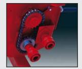
**Reverser Kit** Ability to reverse all flighting. Allows quick and easy clean out (shown with guards removed for clarity).
