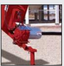
**Right Angle Drive** Assists operation in limited space situations. Allows a full arc on opposite side of tractor.
